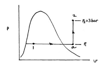
ASSUMPTIONS: 1. The water is a closed system. 2. The pressure is constant until the piston hits the Stops. 3. Priction between the piston and cylinder wall can be ignered. 4. For the system, DPE, DKE can be ignored, 5. g is constant.
